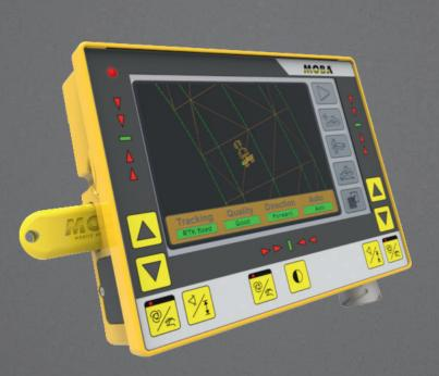
The unbeatable combination of high-end on-board computer and particularly fast controller is a real performance miracle. Together they realize the real-time visualization of the the digital model is the basis for a constant comparison of the terrain with the digital model. In the popular DXF format, terrain models can be easily imported or created on the machine itself.
