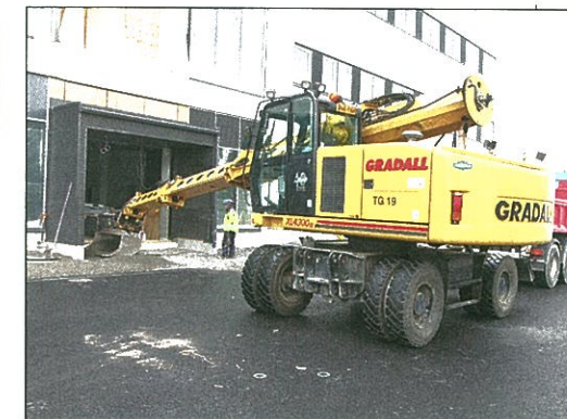
Above and below: Wheeled Gradall excavators equipped with a tilt-rotator result in a machine with a phenomenal working envelope.
