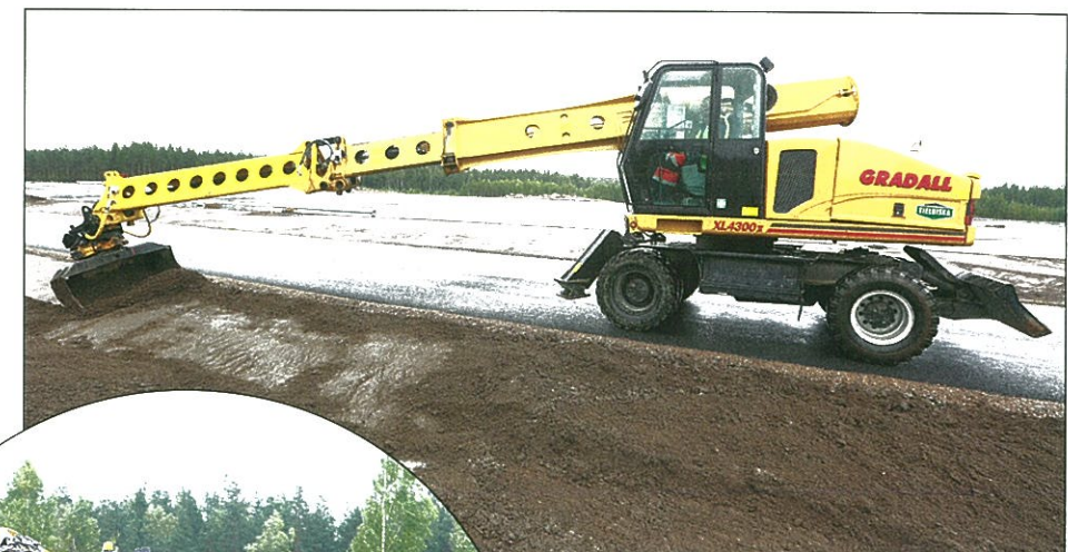
Above and below: Wheeled Gradall excavators equipped with a tilt-rotator result in a machine with a phenomenal working envelope.
