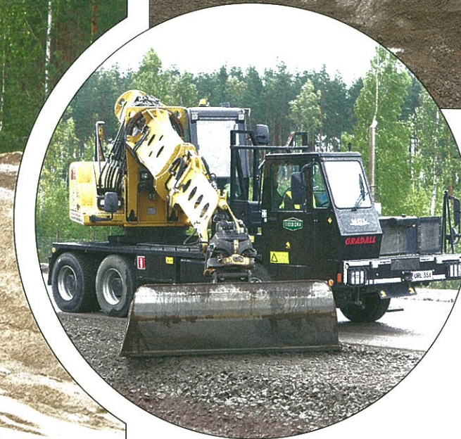
Above and below: Wheeled Gradall excavators equipped with a tilt-rotator result in a machine with a phenomenal working envelope.
